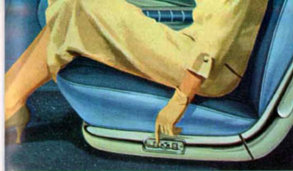
POWER SEAT: Complete six-way adjustment at the touch of your finger—forward, backward, up and down, plus forward and backward tilt for safer, more comfortable driving. Instantly adjustable while driving to cut fatigue on long trips.
