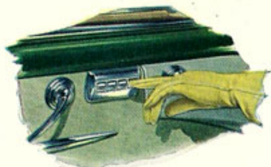
Master Touch —Hydraulic push-button magic permits the driver to raise or lower any side window from his own side of the front seat in his ROADMASTER Riviera or ROADMASTER Convertible.
