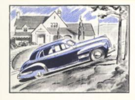
The car may be locked in gear while parked on a steep incline by placing the Hydra-Matic Drive control lever in "R" position after the engine has stopped. This action locks the transmission mechanically when the motor is shut off, making it impossible for the rear wheels of the car to turn.
