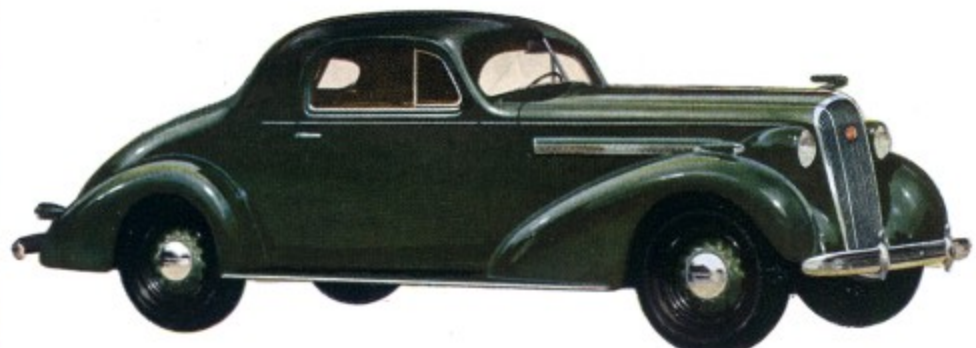
BUICK Series Forty SPECIAL Two-Passenger Business Coupe with deck. 118-inch wheel base. Model No. 46
