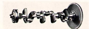
Weighing 71 pounds, this crankshaft of drop-forged high carbon steel is counterweighted and fitted with a vibration damper. Balanced both at rest and in motion, it contributes to smooth, dependable performance.
