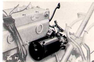
Easy starting is a notable characteristic of the Oldsmobile Six. The starter is the positive engagement type. When you depress pedal, starter gear engages the flywheel before electrical contact is made. Eliminates sticking. Coordination of starter with throttle facilitates starting.
