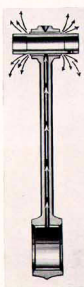
Black lines show how oil is forced, under pressure, to main bearings, connecting rod bearings, piston pins, and camshaft bearings. The connecting rods are rifle-drilled to permit passage of oil, under pressure, to piston pins. A fine car feature, assuring long life and quiet operation.
