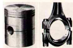
Electroplated pistons permit a close fit and reduce the "breaking-in" period. Connecting rod bearings are the interchangeable thin shell type.
