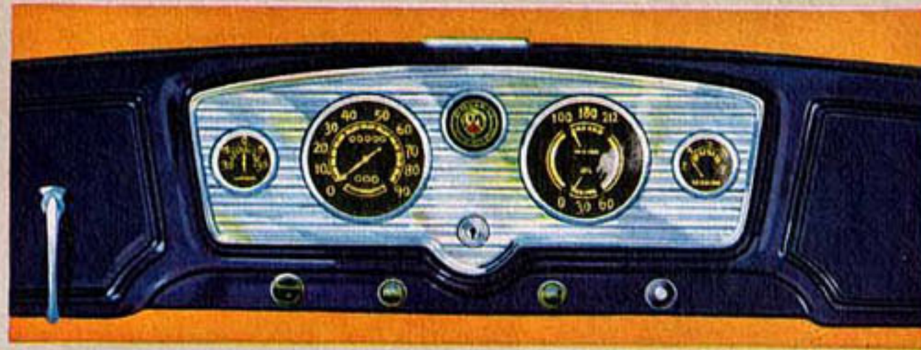
Oldsmobile dial instruments, conforming to latest custom-car practice, are of the full-view "pointer" type, indirectly illuminated. All instruments are clearly visible to the driver.
