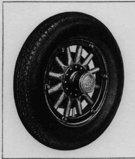
A close-up view of the sturdy wheel and tire. The diameter of the wheel has been reduced, making the spokes short and sturdy. The tire section has been increased so that there is no sacrifice of road clearance. These changes give longer life and massive appearance. The new hub cap is a distinctive feature
