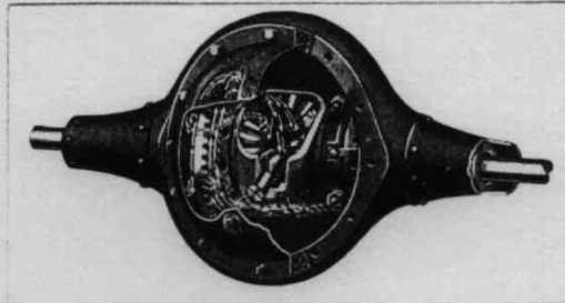
A point typical of Buick's superior construction is apparent in the lubrication of the differential gears. Oil carried up by the ring gear is deflected, by a baffle on the differential housing, directly into the differential gears. Thus positive lubrication is assured at all speeds
