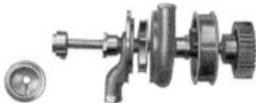
Nickel steel timing gear and shaft that drives fan belt pulley, water pump and magneto.
