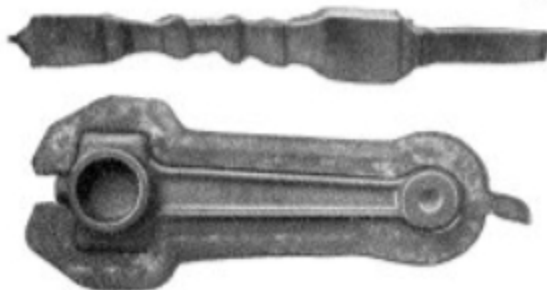
Connecting rod from the first crude shaping after coming from the heating furnace to the finished article.
