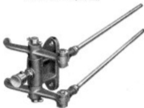
Heat treated valve rocker arms and pins lubricated by grease cup—showing bracket support and cam shaft push rods.
