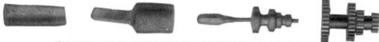
Evolution of a three step nickel steel gear from raw material until ready for heat treating, oil tempering and grinding.
