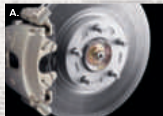
A. To promote linear, fade-resistant stops, power-assisted 4-wheel disc brakes are standard on every MAZDA5, as are an advanced Anti-lock Brake System (ABS) and Electronic Brakeforce Distribution (EBD). B. 4-wheel independent suspension and precise, power-assisted rack-and-pinion steering help endow the MAZDA5 with confidence-inspiring handling. C. The MAZDA5's sophisticated 2.3-liter, DOHC, 16-valve, all-aluminum 4-cylinder engine boasts variable valve timing, 157-hp and responsive performance. D. A slick-shifting 5-speed manual gearbox is standard, while the available 4-speed Sport AT automatic also provides the fun of manually shifting at the flick of a wrist.
