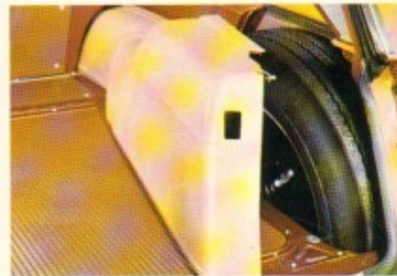
Spare Tire Mounting and Cover. The spare tire is mounted inside the station wagon behind the rear wheelhousing with a swing-out plastic cover for a neat, uncluttered appearance.
