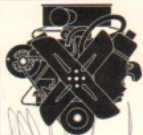
318-cubic-inch V8 Bore: 3.91" □ Stroke: 3.21" □ 2-bbl. carb □ Comp. ratio: 9.2:1 □ Single exhaust □ Power: 230 hp @ 4400 rpm □ 340 lbs.-ft. @ 2400 rpm □ Regular fuel recommended.
