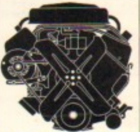
426-cubic-inch Hemi V8 Bore: 4.25" □ Stroke: 3.75" □ Two 4-bbl. carbs □ Un- silenced air cleaner □ Comp. ratio: 10.25:1 □ Dual exhausts □ Power: 425 hp @ 5000 rpm □ 490 lbs.-ft. @ 4000 rpm □ Premium fuel recommended.
