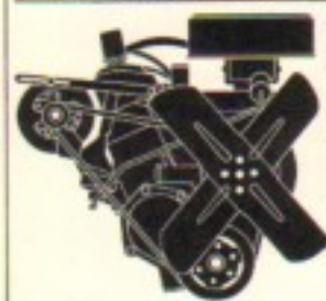
225-cubic-inch Six Bore: 3.4" □ Stroke: 4.125" □ 1-bbl. carb □ Comp. ratio: 8.4:1 □ Single exhaust □ Power: 145 hp @ 4000 rpm □ 215 lbs.-ft. @ 2400 rpm □ Regular fuel recommended.
