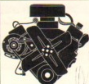
273-cubic-inch V8 Bore: 3.63" □ Stroke: 3.31" □ 2-bbl. carb □ Comp. ratio: 9.0:1 □ Single exhaust □ Power: 190 hp @ 4400 rpm □ 260 lbs.-ft. @ 2000 rpm □ Regular fuel recommended.
