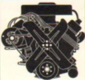
383-cubic-inch V8 Bore: 4.25" □ Stroke: 3.38" □ 2-bbl. carb □ Comp. ratio: 9.2:1 □ Single exhaust □ Power: 290 hp @ 4400 rpm □ 390 lbs.-ft. @ 2800 rpm □ Regular fuel recommended.
