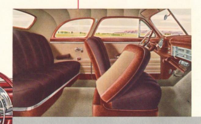
For the driver, everything is within easy reach — in plain sight. Gauges are grouped in the Safety-Eye instrument cluster and can be read easily and quickly at a glance. The directional signal lever at the left, the gear shift lever on the right, and the horn ring can all be operated without taking the hands from the steering wheel. And the engine can be started by merely turning the ignition key.
