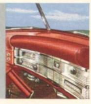
The Chrysler Safety Cushion, extending across the top of the dash panel, is made of thick sponge rubber and covered with leather —a great safety feature.
