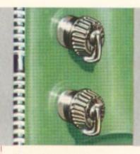
All controls and switches on the instrument panel are a new rotary type—a decided improvement over the old finger stubbing, nail breaking push-and-pull type.
