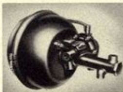
Powerful vacuum brake boosters are available on many models. They reduce driver fatigue and assure greater safety.
