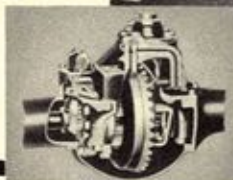
"Dual-Purpose" 2-speed axle models give extra power and hauling ability—economy and fast operation too. With simple finger-tip control, you may pick the gear ratio to fit the load and road. Its economy ratio gives high speed with low engine revolutions. Power ratio gives real "lugging ability" for heavy hauling.
