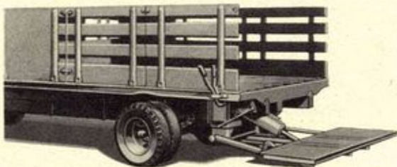
Elevating tail gates, operated hydraulically or mechanically, are available in several varieties to buyers of these trucks.
