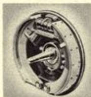
Powerful, "equal-pressure" hydraulic 4-wheel brakes assure safe, sure, smooth stops.
