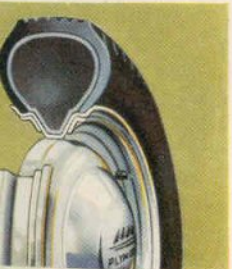
Rim Wheels hold tires in position on rim in case of a flat, insure safer stopping.
