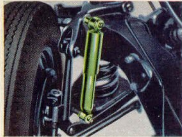
Airplane-Type Shock Absorbers cushion and control spring action at all four wheels for maximum comfort.
