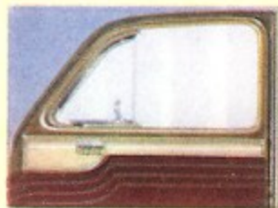
Detail, showing how the plastic door moulding forms a continuation of the instrument panel.
