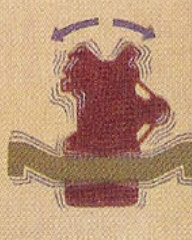
Floating Power mountings are low at the rear of the Plymouth engine.
