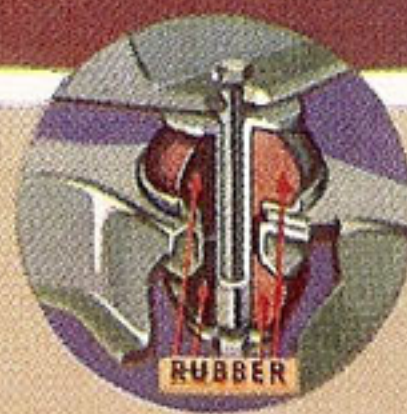
Floating Power mountings are low at the rear of the Plymouth engine.
