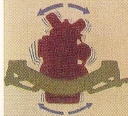
With most of the engine weight above the mountings (right) vibration is intensified and transmitted to frame and body of a car. With Floating Power (left) the weight below the center of balance resists movement by the equal weight above and the power impulses result only in a gentle rocking motion.
