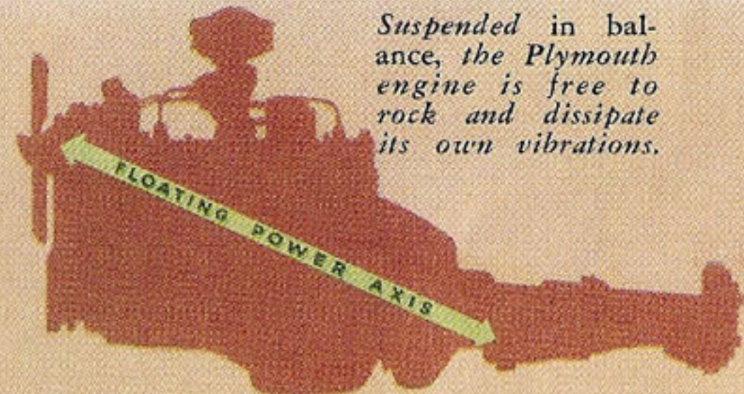
Floating Power mountings are low at the rear of the Plymouth engine.
