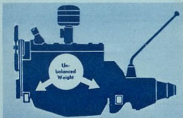
OLD WAY —with nearly all engine weight above the mountings, resulted in top-heaviness, aggravated the vibrations which always occur in every automobile engine as a result of its power impulses.
