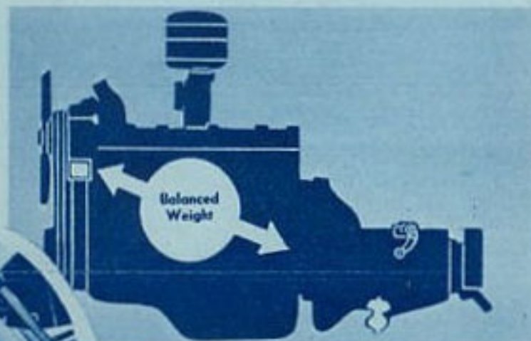
FLOATING POWER! High at the front, low at the rear, Floating Power mountings suspend the Plymouth engine in balance .
