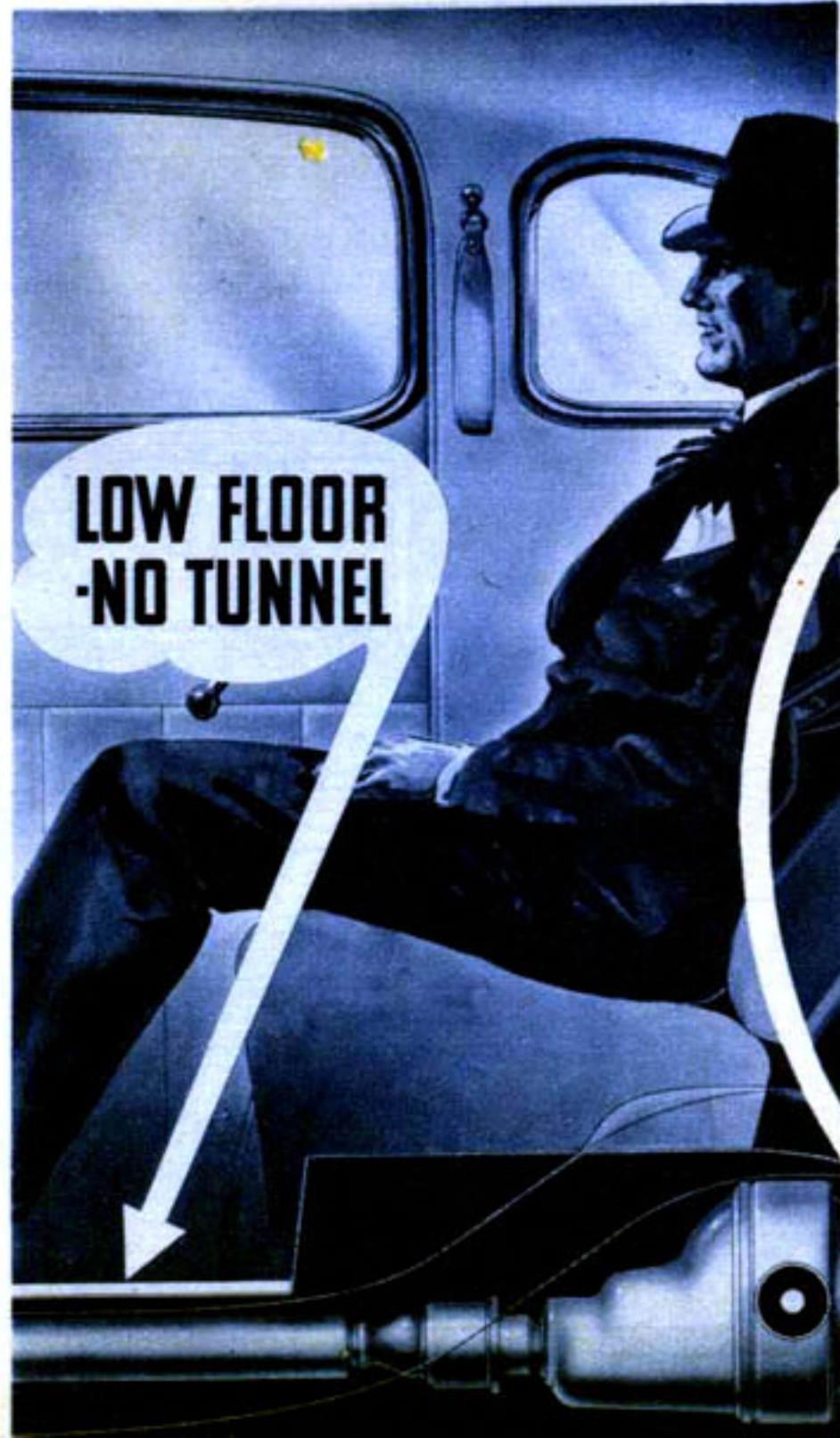
With no tunnel in the floor, the center passenger in Plymouth's deep, wide rear seat rides as comfortably as those on either side. Absence of rear compartment floor tunnel is made possible by use of the new hypoid rear axle which lowers the driveshaft, making a tunnel unnecessary.
