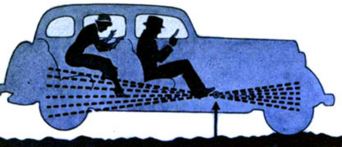
The old way. Stiff front springs and 60 per cent of weight on rear springs caused front end bounce.
