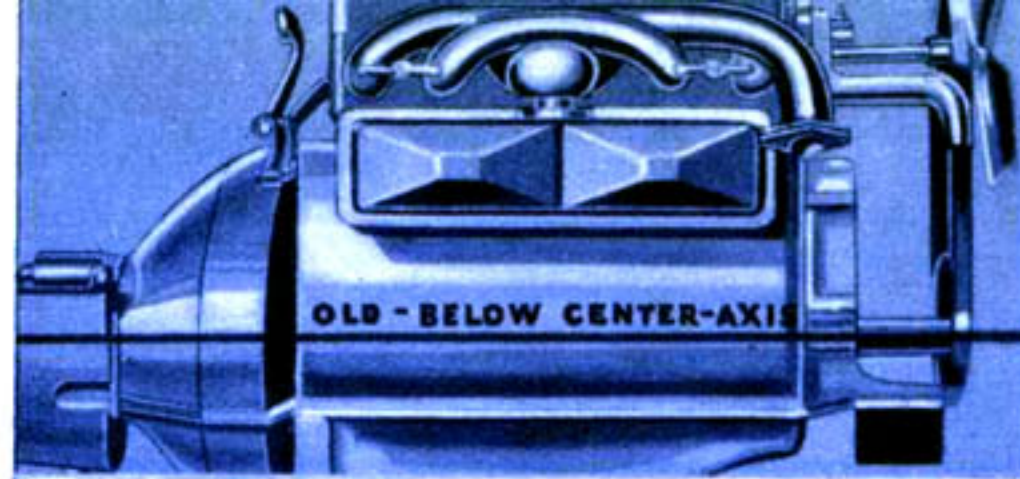
The old-way—engine top-heavy on its mountings—it increased the tendency to vibrate.
