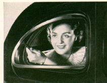
Simplified! The rear window ventilator operates by this simple latch, eliminating bulky mechanism.
