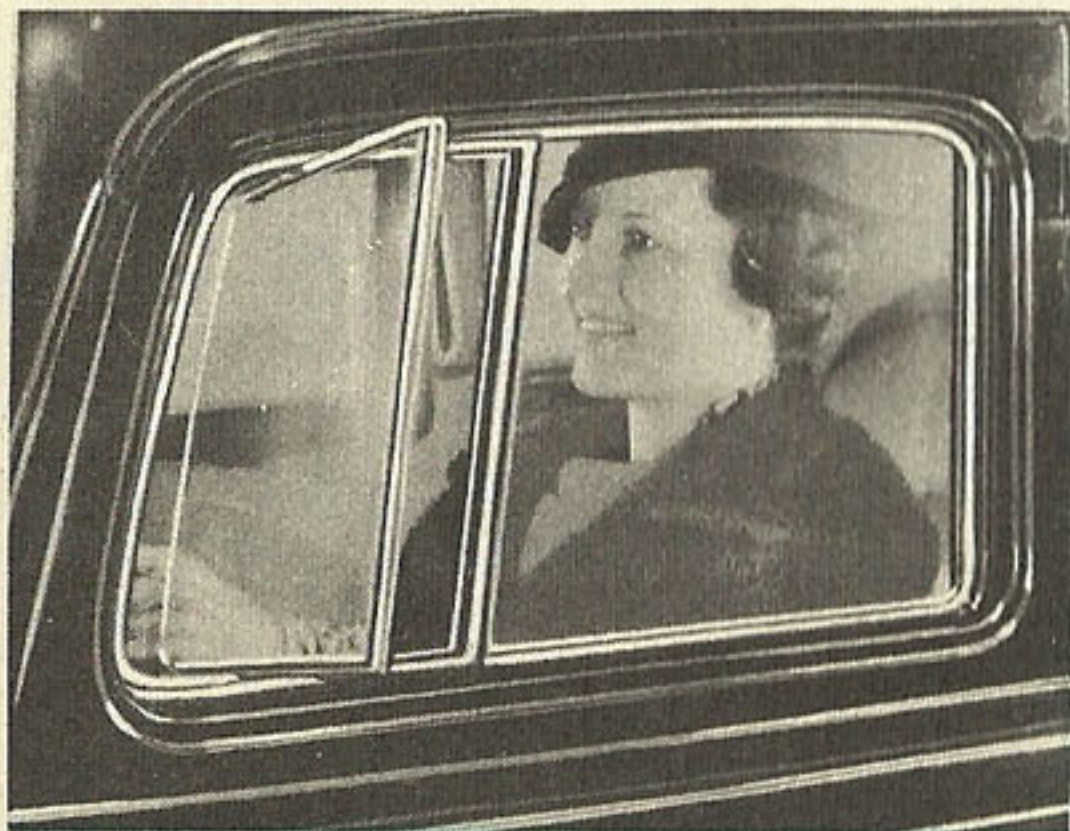
With the front ventilator partly open air currents create a partial vacuum behind the glass which gently withdraws stale air.
