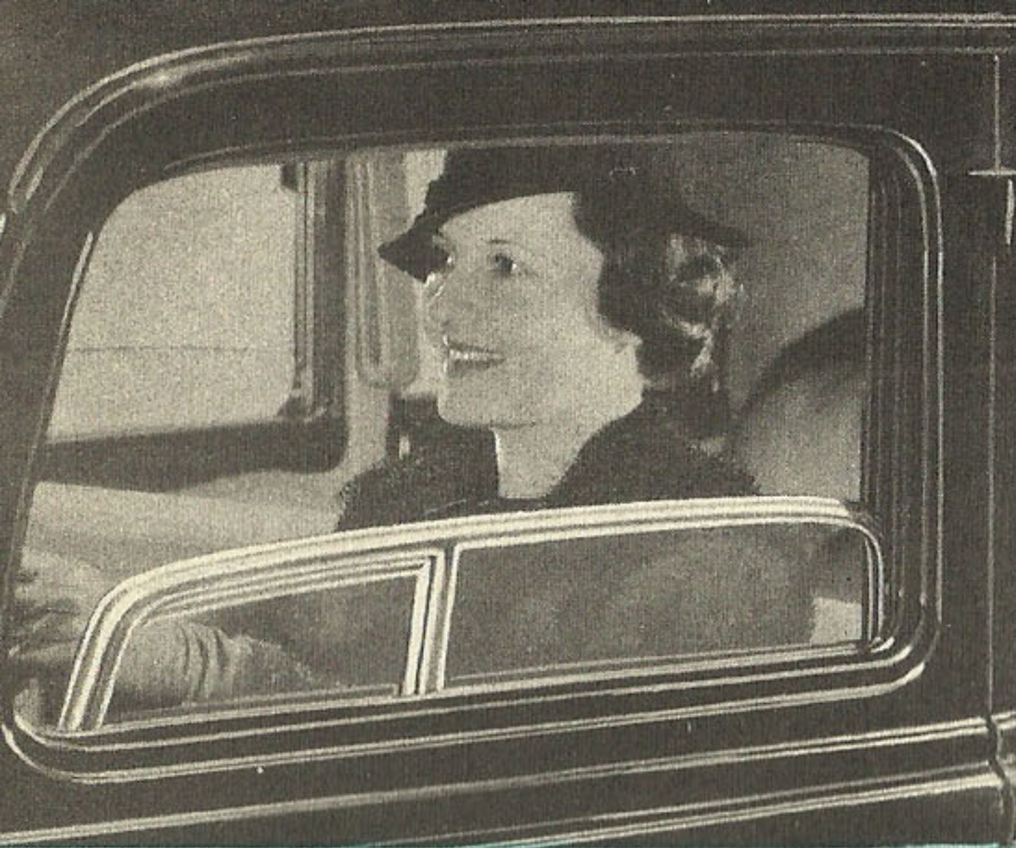
The entire front window can be lowered as a unit affording complete ventilation without obstructions.
