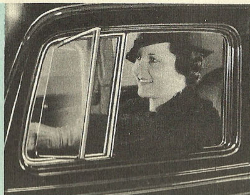
Front ventilators may be set to literally scoop in fresh air and if desired rear half of window may be lowered to secure additional ventilation.
