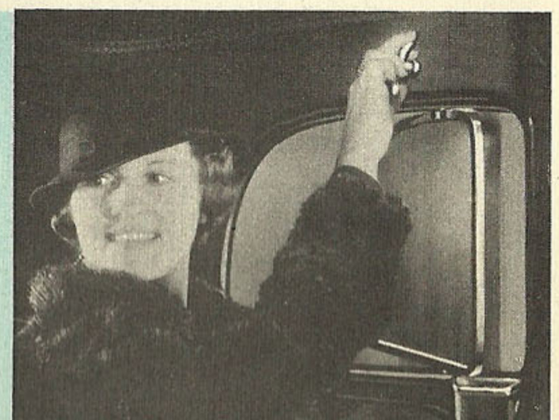
The rear quarter window is rotated on its pivots by a control conveniently located above the window where it is accessible yet out of the way.
