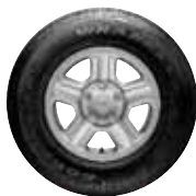
16-inch Slot Spoke Styled Steel painted Argent Standard on Wrangler X and Wrangler Unlimited X
