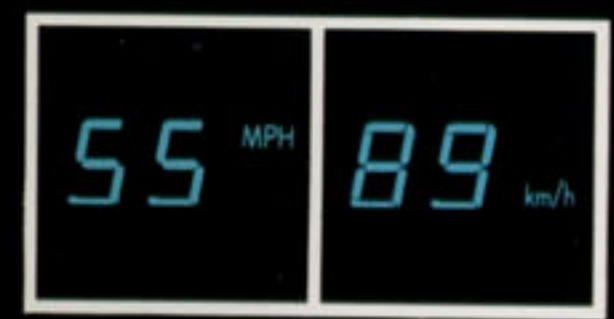
1. Mode-U.S. Met. At a touch converts reading on speedometer, odometer and fuel displays from U.S. to metric or vice versa.
