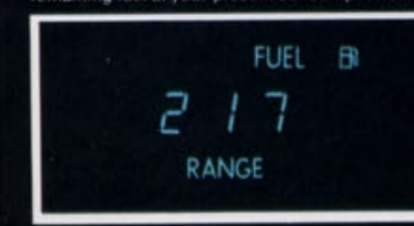
6. Fuel-Range. Pushing the button displays estimated number of miles that can be driven on remaining fuel at your present consumption rate.
