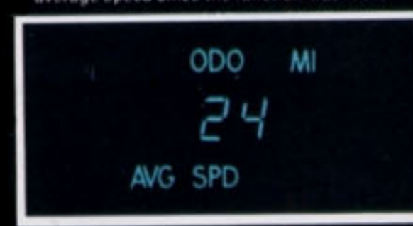
5. Odometer-Avg. Spd. Shows car's total accumulated miles. Push button to display car's average speed since the function was reset.
