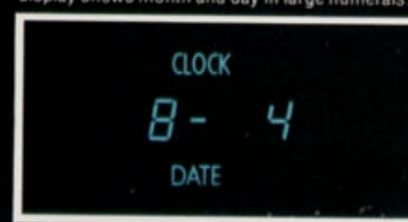
2. Clock-Date. Shows time of day in large numerals, and AM or PM. Push button and display shows month and day in large numerals.
