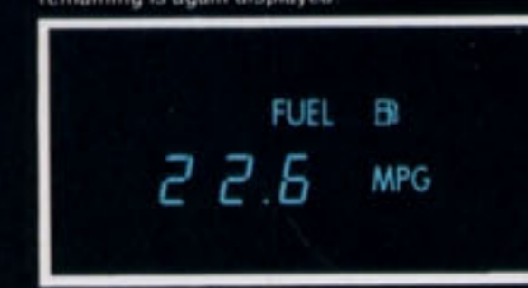
7. Fuel-Present. Displays the fuel consumption rate (MPG) which is recalculated every two seconds. When button is re-touched, fuel-remaining is again displayed.
