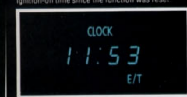
3. Clock-ET. Pushing the ET button replaces time of day with the number of hours and minutes of ignition-on time since the function was reset.
