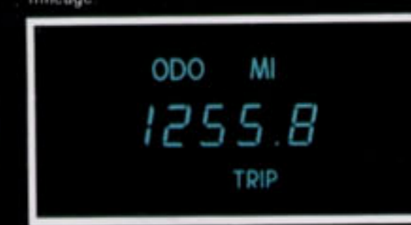
4. Odometer-Trip. Touch of button reveals distance since trip odometer was last reset to ZERO. A second push displays the car's total mileage.
