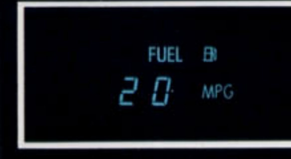
8. Fuel-Trip. Pushing the FUEL-TRIP button displays the MPG consumption since the FUEL-TRIP function was last reset to ZERO.
