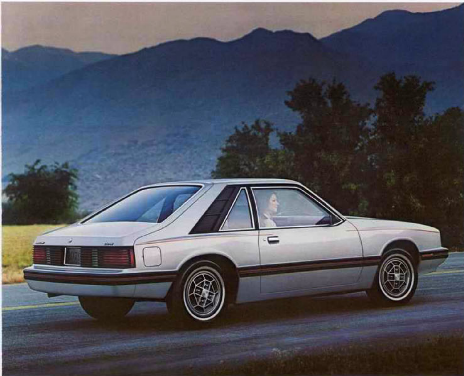
Capri standard equipment: 2.3 litre engine; 2-V carburetor; 4-speed, floor-mounted manual shifter; rack-and-pinion steering; advanced strut front suspension; front stabilizer bar; front disc brakes; four-bar link rear suspension with coil springs; color-keyed bumpers; bright drip moldings; wraparound bodyside molding, and black simulated quarter louvers. Optional sport wheel covers, 14 inch wheels, white sidewall tires, electric rear window defroster and license frame are also shown here. See Pages 12 and 13 for additional options.
