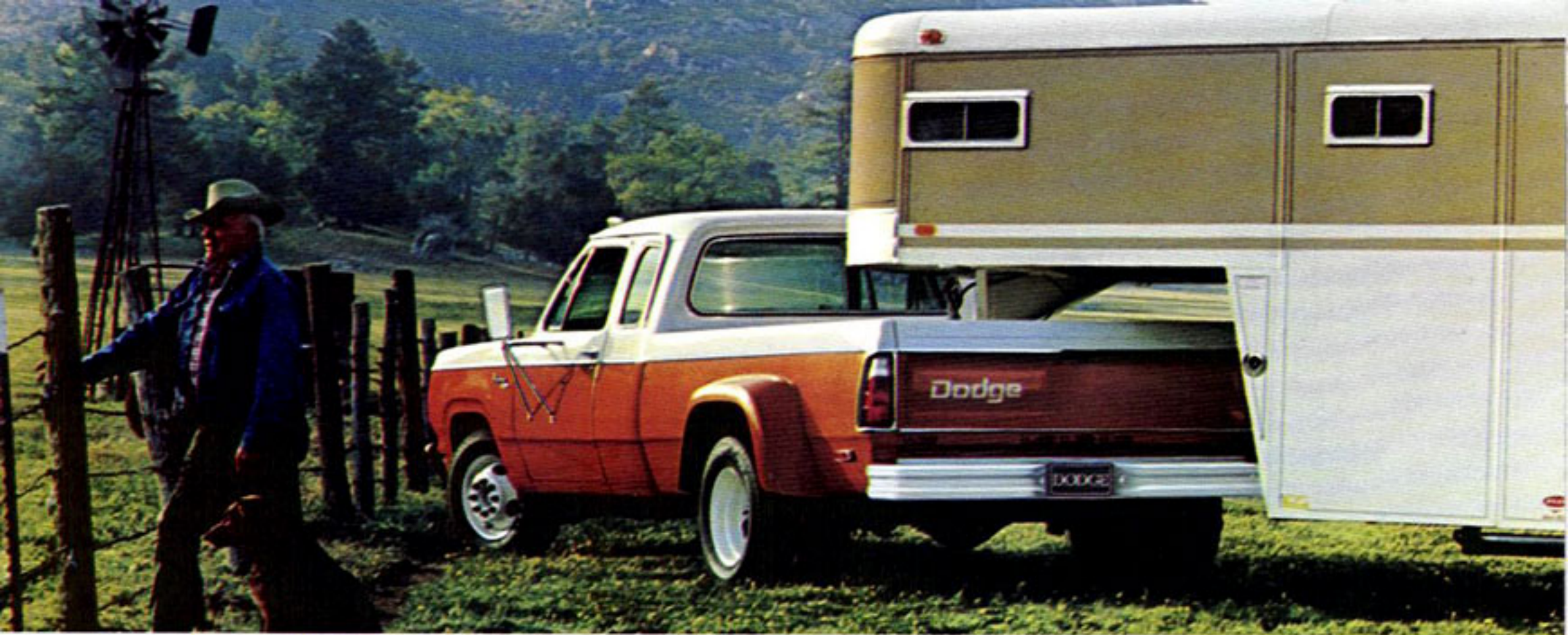
DYNA-TRAC, with dual rear wheels and 10,000-pound GVW. Shown above, D300 Adventurer Sweptline with Dyna-Trac. With optional step-type bumper and rear vision mirrors.
