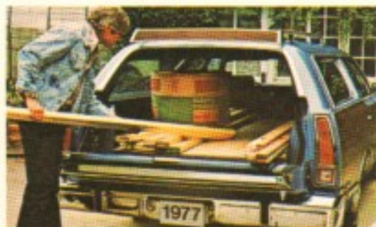
The Marquis three-way tailgate affords extra platform length when dropped level with load floor and facilitates loading.
