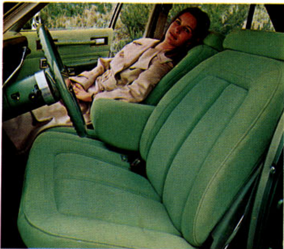
Volaré Premier's optional 60/40 cloth bench seat with center armrest and dual seat-back recliners.
