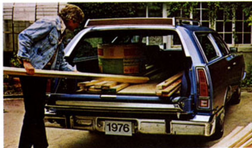
The Marquis and Montego three-way tailgate affords extra platform length when dropped level with load floor. It facilitates loading and unloading, even 4' x 8' panels.
