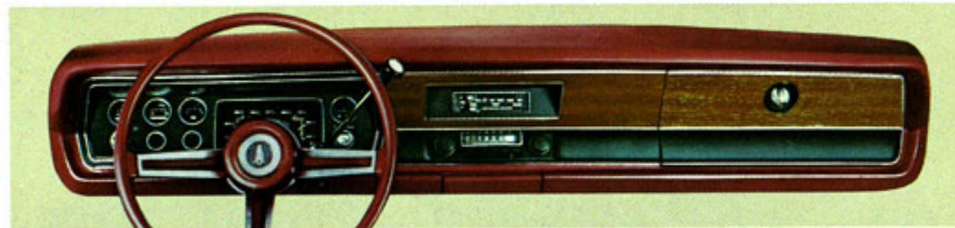
Duster instrument panel with easy-to-read dials shown with optional decor dress-up trim.
