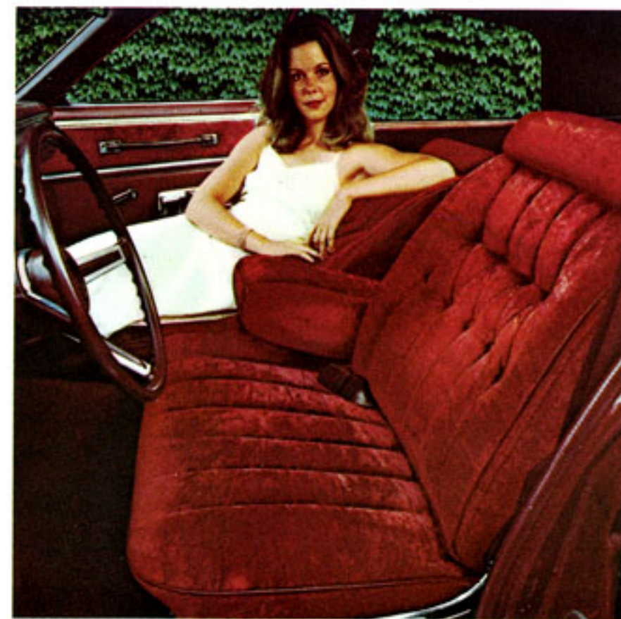
Salon optional velour cloth-and-vinyl 60/40 bench seat with folding center armrest and dual reclining seat-backs.
