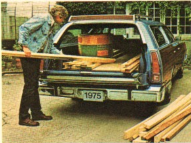
The drop gate of the three-way tailgate affords extra platform length flush with load floor. It facilitates loading and unloading, even bulky 4' x 8' panels.
