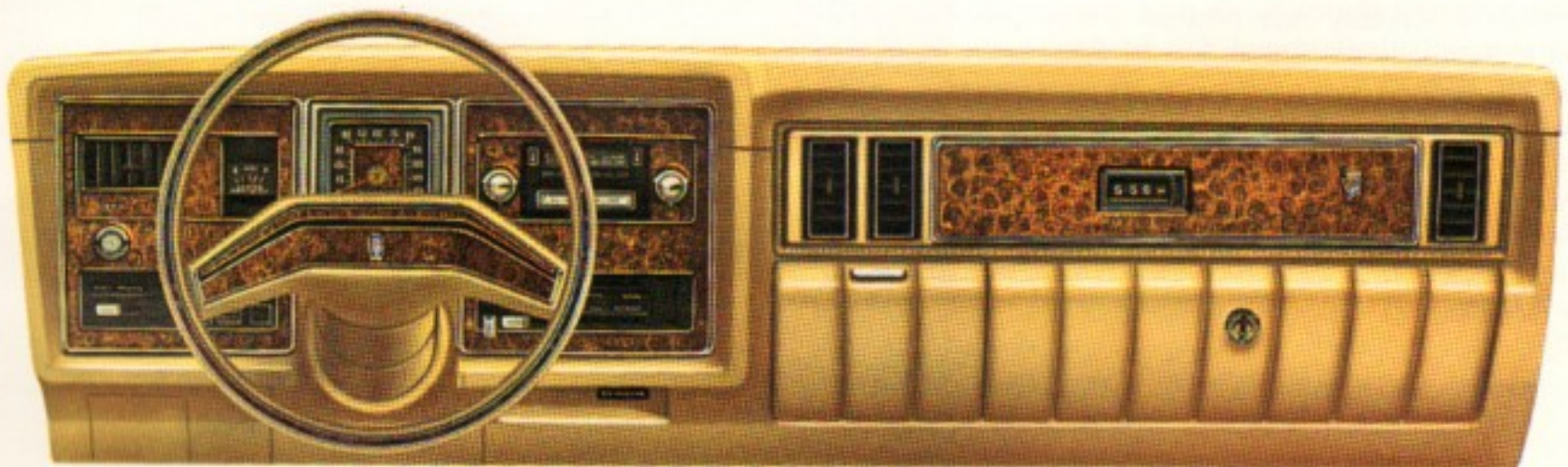
Monarch Ghia instrument panel with optional AM/FM stereo tape, air conditioning and automatic transmission.
