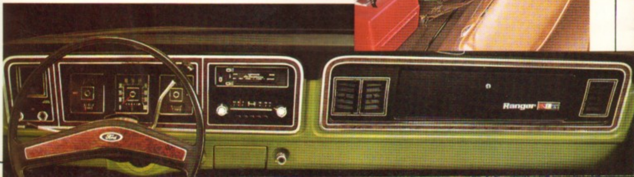
Ranger XLT instrument panel shown with optional air conditioner, SelectShift Cruise-O-Matic and push-button radio.
