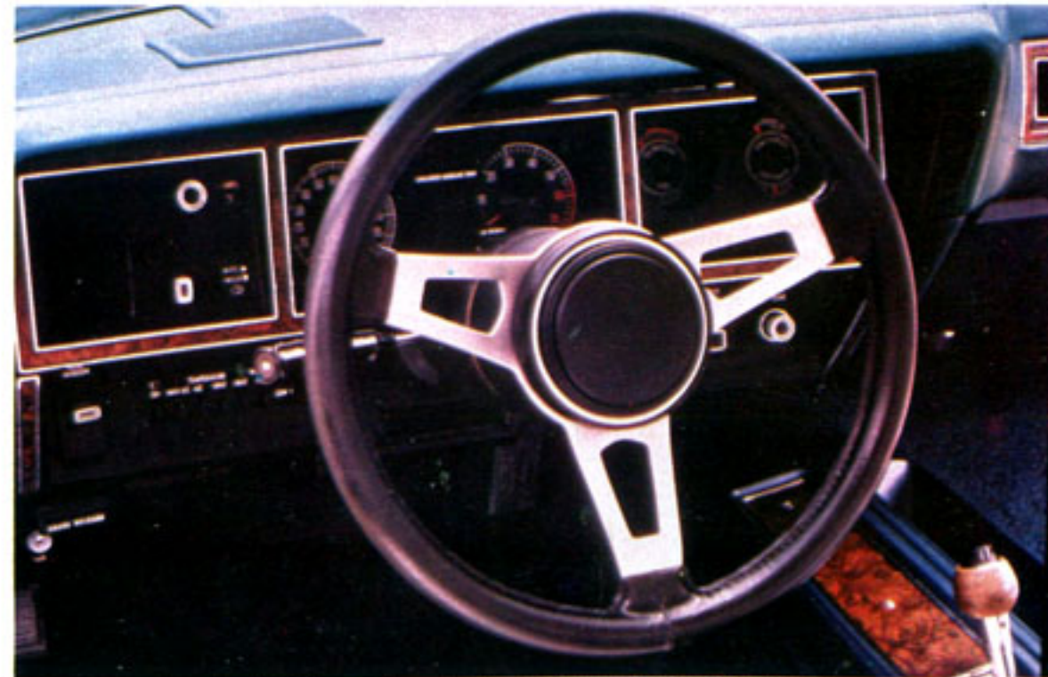
Instrument panel with optional "tach" and "Tuff" steering wheel.
