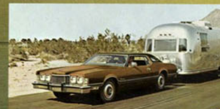
Trailer Towing Package. Thunderbird's quiet, even-keel ride, so relaxing on long trips, stems from its advanced suspension design. The Trailer Package lets you tow up to 6000 lb. gross weight, 700 lb. tongue load. It includes a heavy-duty suspension, extra-cooling package with coolant recovery system, 70-amp. alternator, wiring harness, towing decal, high ratio axle.
