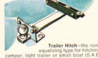
camper, light trailer or small boat (S.A.E. Class I-2000 lbs.) (NOTE: Use with proper Trailer Hitch Ball).
