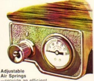
—provide an efficient means of obtaining variable support for improved riding and handling when carrying heavy rear-end loads. They are recommended for Cougars, Montegos and Cyclones towing light weight loads (control illustrated).
