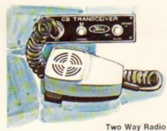
—a 12 channel transceiver that can be converted to Base Station with the addition of power supply (not illustrated). Also available for 12 channel unit is a power supply recharge battery and a tone alert (not illustrated).
