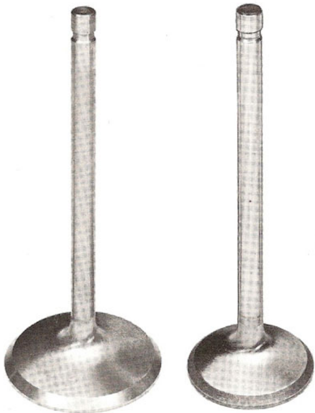
Lightweight Titanium Intake Valve (DOZX 6507-A) On Left, Lightweight Exhaust Valve (DOZX 6505-A) On Right.
