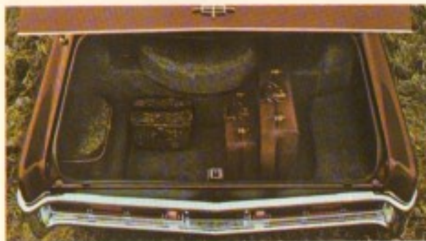
Continental's luggage compartment has a usable capacity of 18.1 cubic feet, fully carpeted. An optional remote-control duck-lid release includes a trunk-open warning light on the instrument panel. The tire cover is also optional.
