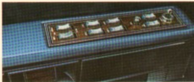
Padded armrest on driver's door organizes switches (left to right) for window and door locks, four power windows, power sun control and remote-control outside mirror. A lighted, concealed ashtray and an individual window control are designed into each of the three passenger armrests.
