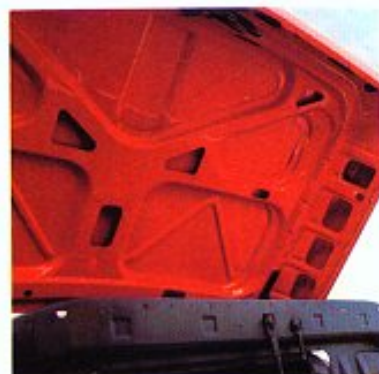
Double-wall section hood strength
