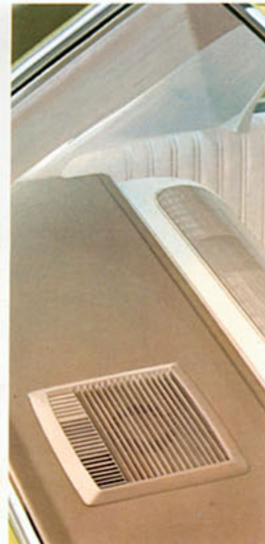
Rear Window Defogger. Directs stream of air on glass to help keep rear window clear for better visibility.
