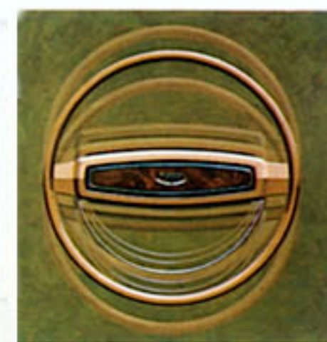
Tilt Steering Wheel. May be tilted vertically to any one of seven driving positions for more comfortable, more efficient driver control, or tilted to uppermost position for ease of exit or entry.
