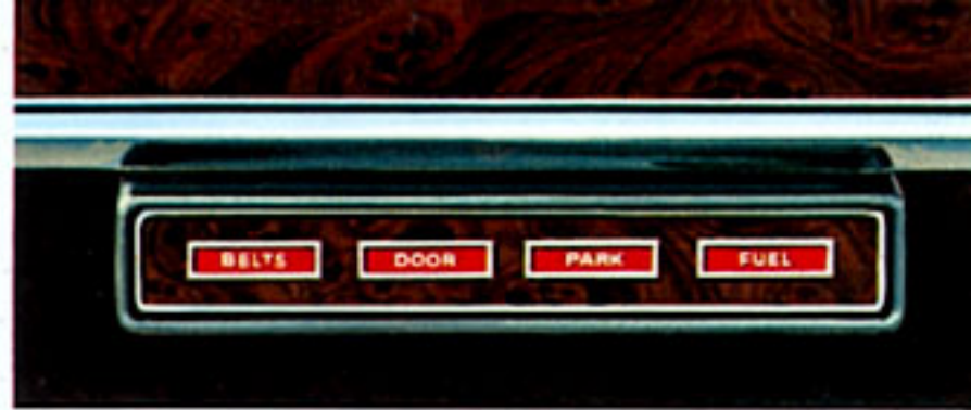
Convenience Group has warning lights for door ajar, low fuel, parking brake and to fasten seat belts.
