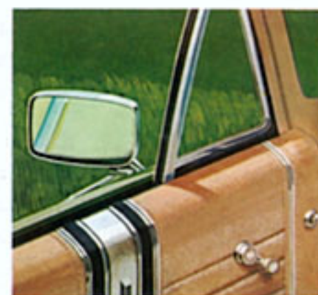
Remote-Control Outside Mirror Can be adjusted conveniently from inside by the driver. Available in Visibility Group option, or as separate option.
