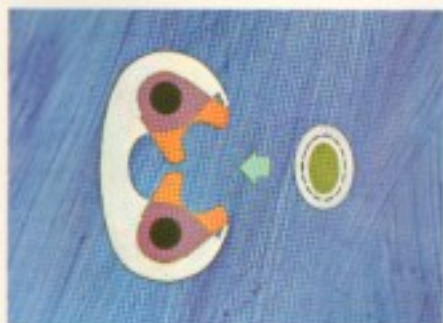
Double-Yoke Safety Door Latches and Safety Hinges are strong, tight-gripping to help keep doors closed in event of impact. (Safety-Rotor type on Club Wagons.) As an added precaution, Positive Door Lock Buttons must be raised before door handles will operate and doors can be opened.
