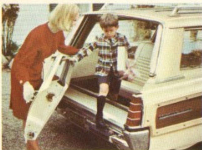
In this illustration, Mercury's tailgate is swung out as a rear door for easy passenger entrance and exit from the rear.
