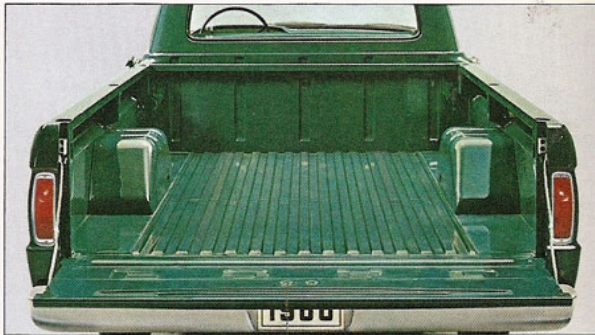
EXTRA-STRONG TAILGATE. Sturdy double-wall tailgate with heavy steel hinge-type straps is strong enough to support a ton load in the open position. To lower the tailgate for close-in loading, straps are easily detached from the tailgate.
