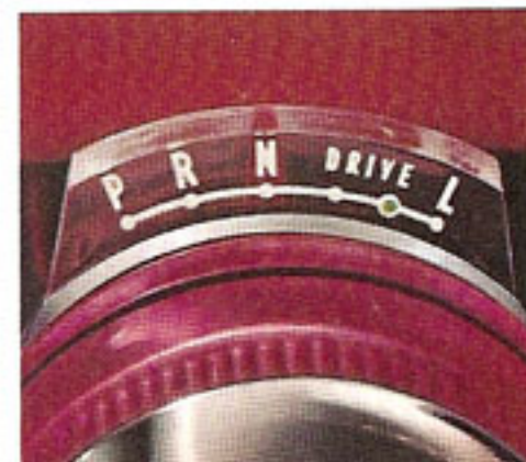
Cruise-O-Matic transmission is fully automatic and has two selective forward drive ranges.
