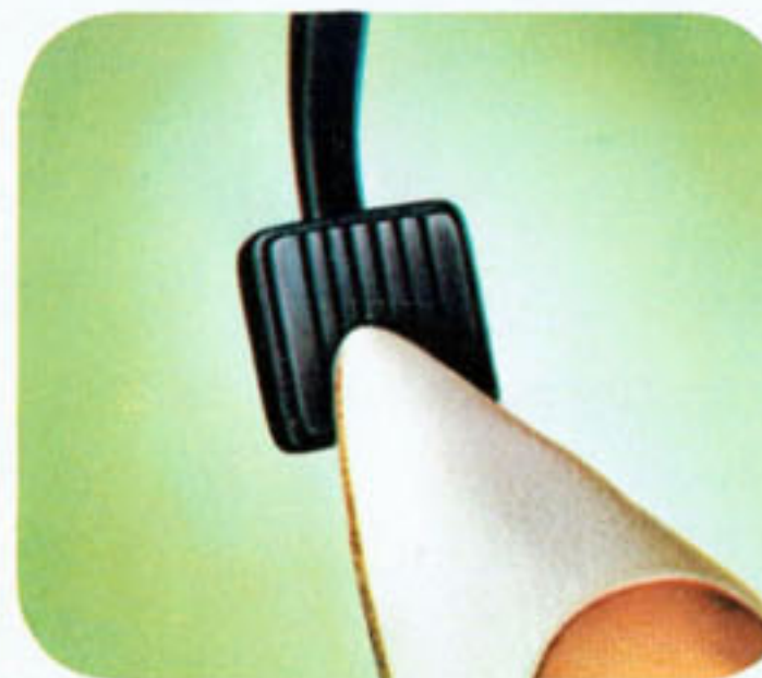
New foot-operated parking brake
