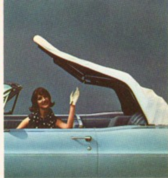
New convertible top is constructed of rugged 5-ply satin finish vinyl for durability. Glass rear window (standard) resists scratching, discoloring and can't wrinkle. Power top is optional.
