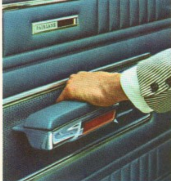
Combination safety (red) and courtesy (white) light mounted in front arm rests are standard on XL and GT models. Door panels are luxurious vinyl with bright trim moldings.
