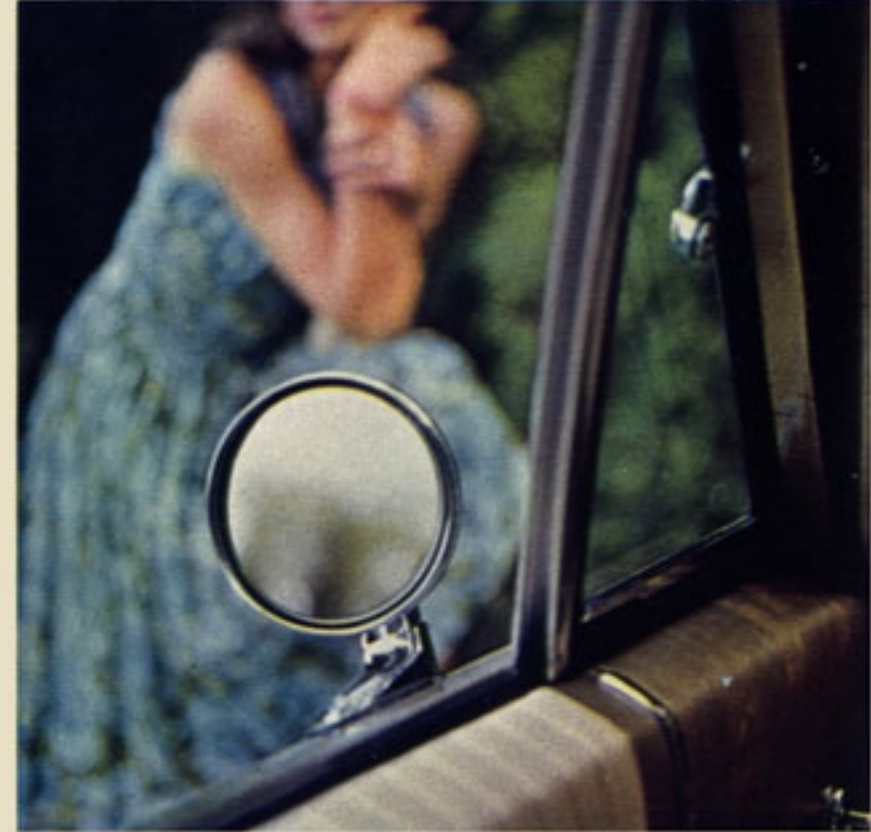
Aim outside mirror accurately and simply, without opening window, by adjusting control lever on inside of door panel.
