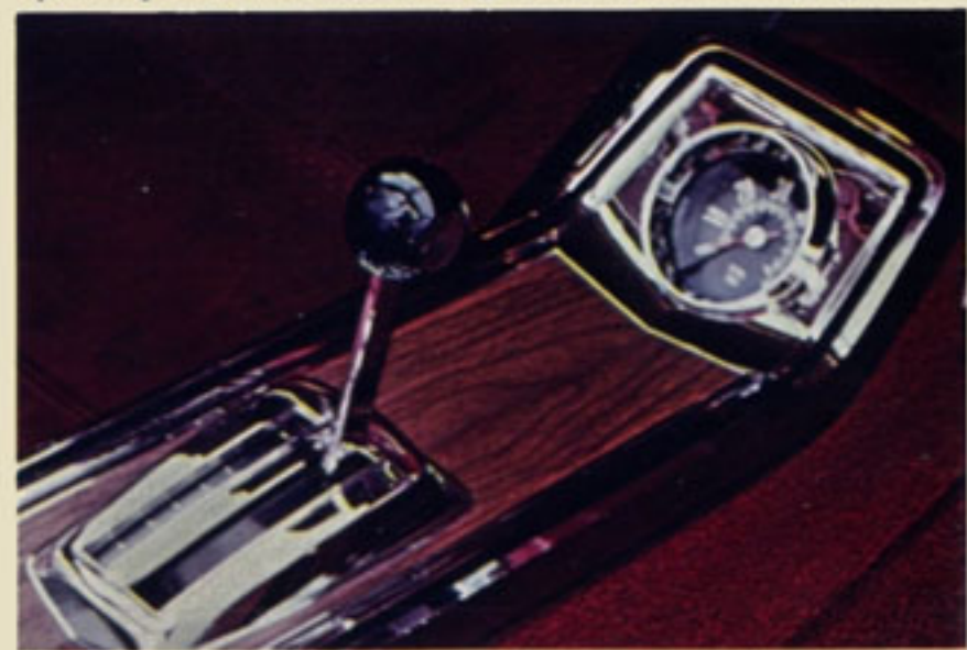
Console-mounted automatic transmission with Hurst linkage
