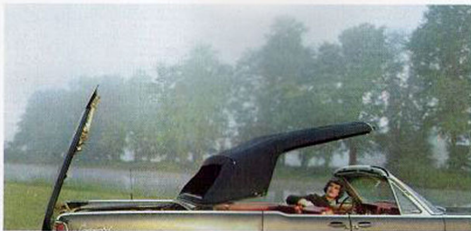
The weather-resistant top stores completely within the rear deck. When the top is raised, power locks secure it to the windshield, automatically.
