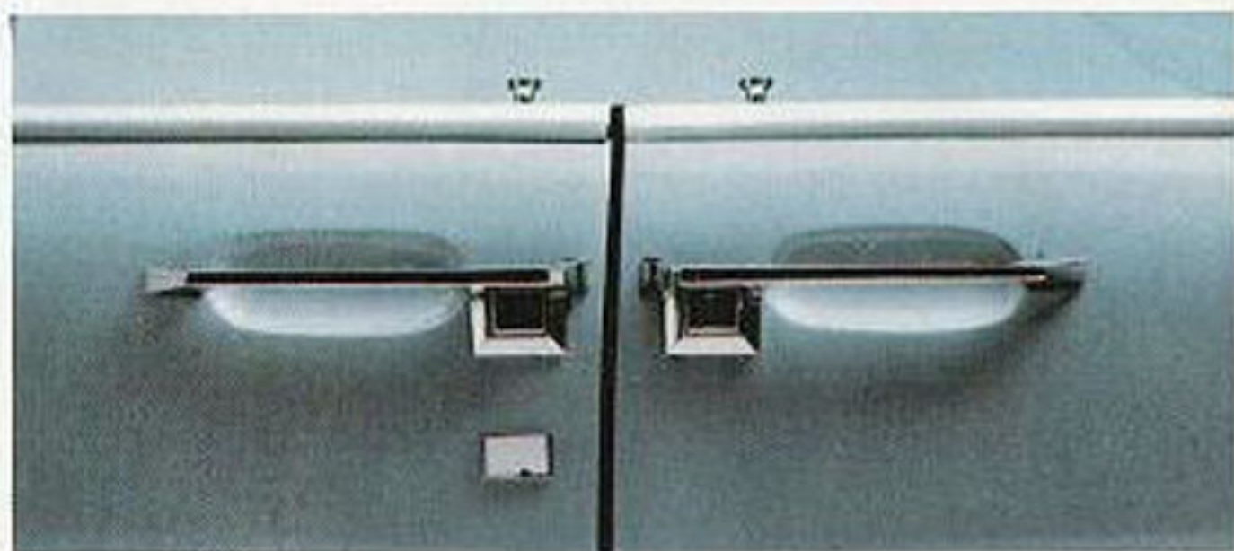
Lincoln Continental's center-opening doors feature power-operated door locks—activated by an instrument panel switch.
