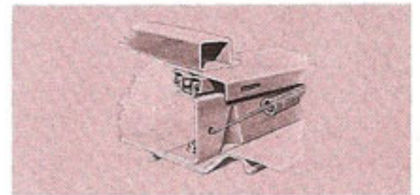
NEW SEAT ANCHORAGE . . . front seat glides on 12 steel balls for easier 5\frac{1}{2} " 11-position adjustment, smoother operation. Positive safety stops in each inclined seat track resist separation from undue force of impact.
