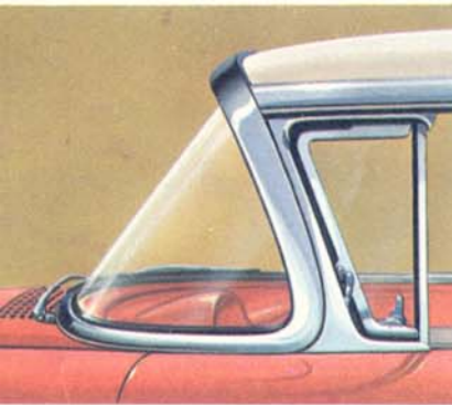
A silver crown of stainless steel slants out over the windshield top for greater strength and glare protection. New rain shields on front door protect the inverted-triangle vent windows.
