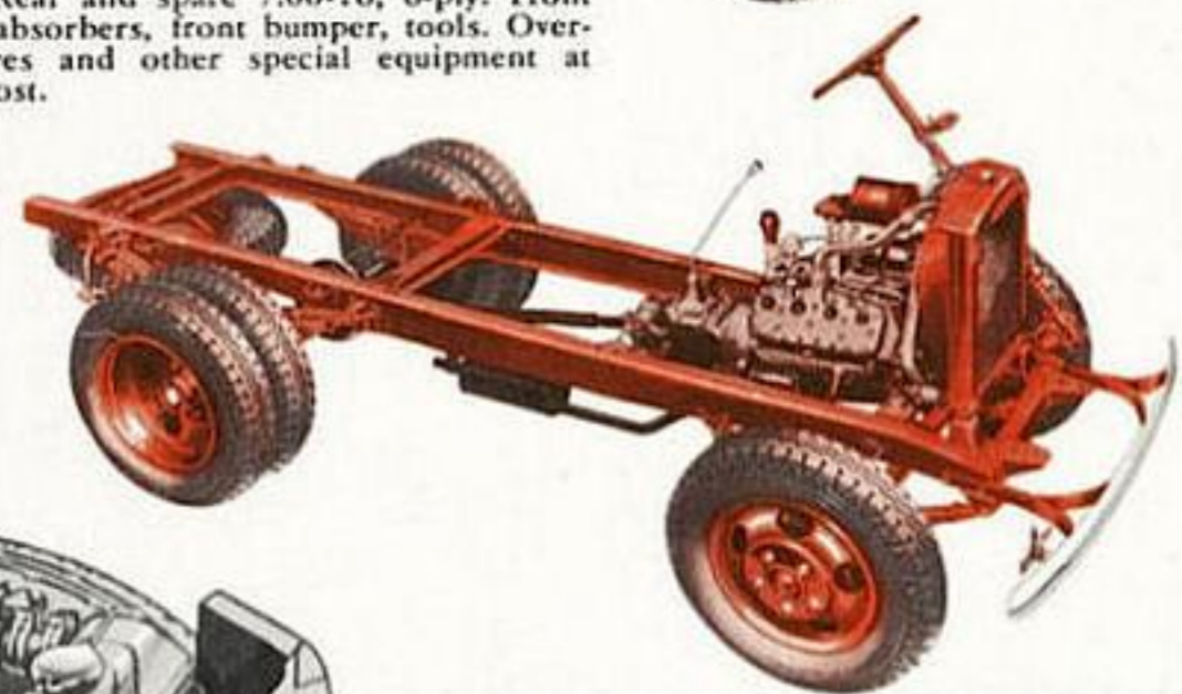
101 INCH C.O.E. CHASSIS (85 or 95 hp) Standard equipment: Cab, hood, front fenders; running boards; instrument panel; horn; lamps. 23 gallon fuel tank; spare wheel carrier; five wheels. Tires: Front 6.00-20, 6-ply. Rear 6.50-20 (32 x 6) 8-ply. Front bumper; jack and tool kit. Dual wheels, heavy-duty tires, auxiliary springs, two-speed axle, frame reinforcements and other special equipment available at additional cost.
