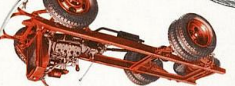
122 INCH CHASSIS (85 hp V-8 or 4-cyl) Standard equipment: Hood, cowlf, front fenders, running boards, instrument panel, horn, lamps, front bumper, tools. Over-6-ply, Rear and spare 7.00-16, 6-ply, Front spare 7.00-17, 6-ply, \frac{1}{2} -ton—Front 6.50-16, One-Ton—Front 6.00-17, 6-ply, Rear and spare 7.00-17, 6-ply, \frac{1}{2} -ton—Front 6.00-20, Rear 6.50-20 (32 x 6) carrier; five wheels. Tires: Front 6.00-20, Rear 6.50-20 (32 x 6). Standard equipment: Hood, cowlf, front fenders, running boards, instrument panel, horn, lamps, front bumper, tools. Over-6-ply, Rear and spare 7.00-16, 6-ply, Front spare 7.00-17, 6-ply, \frac{1}{2} -ton—Front 6.50-16, One-Ton—Front 6.00-17, 6-ply, Rear and spare 7.00-17, 6-ply, \frac{1}{2} -ton—Front 6.00-20, Rear 6.50-20 (32 x 6) carrier; five wheels. Tires: Front 6.00-20, Rear 6.50-20 (32 x 6). Special equipment available at additional cost.
