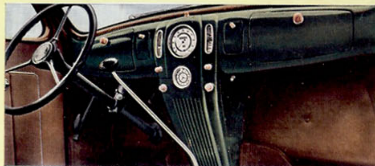
Notice the electric clock, and the two glove compartments. A radio speaker and heater may be installed behind the grille under the instrument panel.
