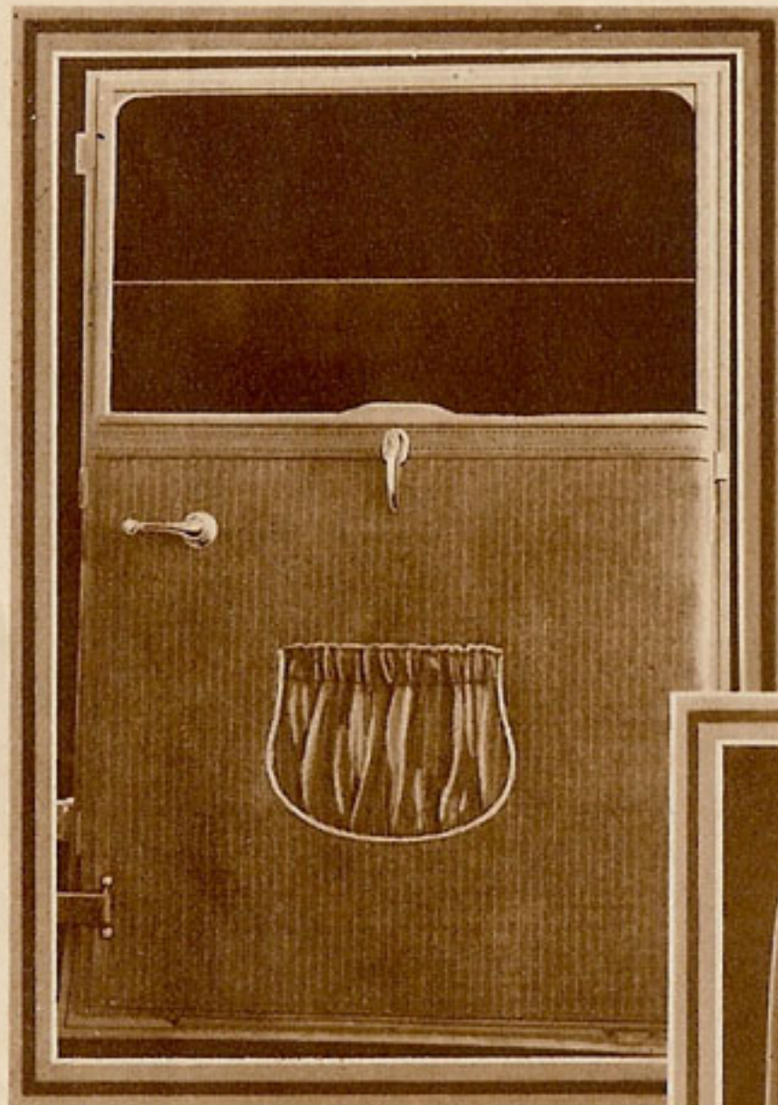
Showing inside of coupe door with lace trim, gathered pocket, revolving window lift and remote control for door lock. Window glass lowers flush with sill.
